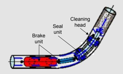
All units have openings that allow the entire fluid flow of a pipeline to bypass. The brake unit ensures that  $\mathsf{HAPP}^{\mathsf{TM}}$  is held back against the fluid flow in the pipeline. Thus the fluid pushes against the following seal unit which channels it into the openings of the cleaning head.
